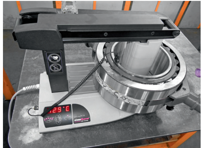
The roller bearing placed around the coil of an IH 210 heater is heated by induction. A simatool Bearing Handling Tool is in place to simplify positioning the bearing on the shaft, once the specified mounting temperature is reached.
